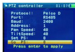
PTZ control set-up
